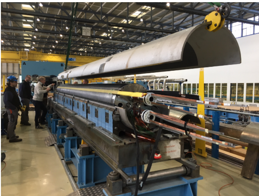
11T dipole ( \text{Nb}_3\text{Sn} ): long prototype under assembly at CERN (Bldg 180 Facility)
