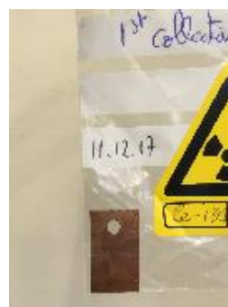
149/152/155/161Terbium ions collected in metal foils
