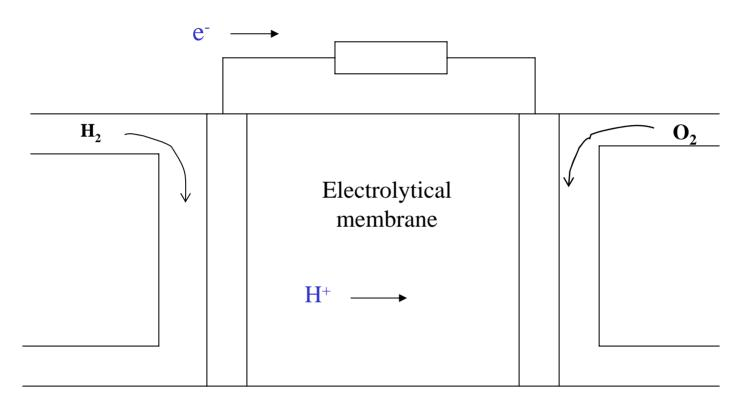
Anode Cathode Reaction:  $H_2 = 2H^+ + 2e^ O_2 + 4H^+ + 4e^- = 2H_2O$  $J = 200 - 500 \text{ mA/cm}^2$ , V = 0.6 - 0.8 V
