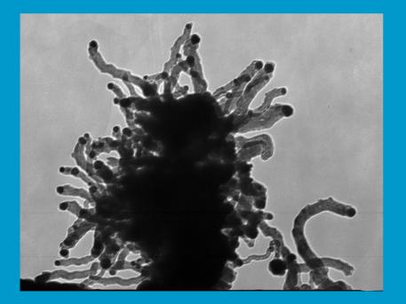
Transmission electron microscopy image of carbon nanotube composite with Ni nanoparticles (dark spots )
