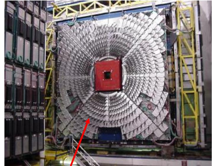
Forward Muon Scintillators System
