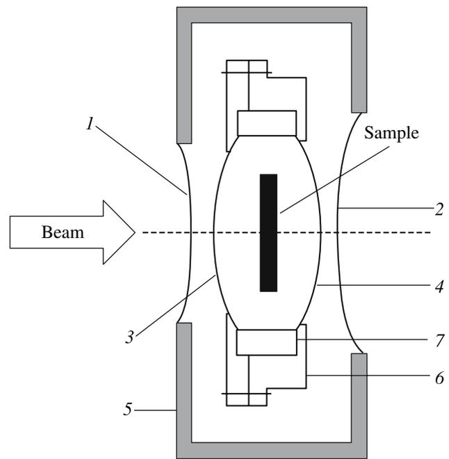
**Fig. 2.** Cryostat and location of a sample in the cryostat for  $\mu$ SR investigations: (1, 2) entrance and exit hot windows, respectively; (3, 4) entrance and exit cold windows, respectively; (5) cryostat casing; (6) beryllium bronze chamber of the cryostat; and (7) sample holder.
