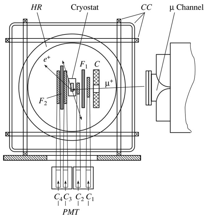
**Fig. 1.** Setup for the  $\mu$ SR experiments: (*HR*) Helmholtz rings, (*CC*) compensating coils, (*C*) collimator, (*F*<sub>1</sub>, *F*<sub>2</sub>) filters, (*PMT*) photomultiplier tube, and (*C*<sub>1</sub>–*C*<sub>4</sub>) scintillation counters.
