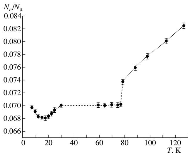
**Fig. 4.** Ratio of the integrated yield of positrons to the total muon number  $N_e/N_\mu$  as a function of temperature  $T$  for alloy  $\text{Fe}_{0.54}\text{Ni}_{0.28}\text{Cr}_{0.18}$ .
