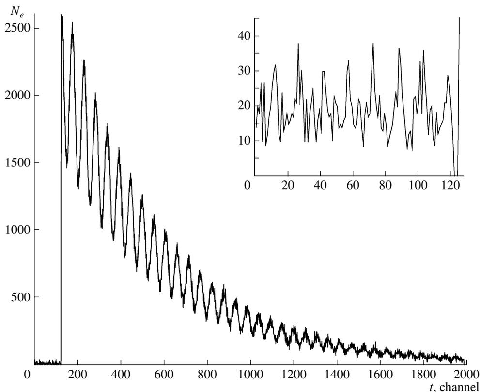
**Fig. 5.** Example of the original  $\mu\text{SR}$  spectrum obtained for the 40-mm-diameter 5-mm-thick copper sample in the transversal (with respect to the spin direction) external magnetic field with induction  $B = 278$  G at temperature  $T = 300$  K. The background distribution in the interval from the origin of the converter scale to the time zero is shown in the inset. One channel on the horizontal scale (time  $t$ ) corresponds to 5 ns, and the time zero is in the 126th channel.
