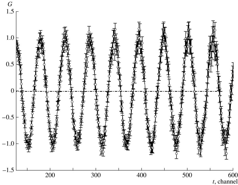
**Fig. 6.** Function of spin relaxation in the transversal (with respect to the muon spin direction) external magnetic field with induction  $B = 278$  G for the 40-mm-diameter 5-mm-thick copper sample at temperature  $T = 300$  K. One channel on the horizontal scale (time  $t$ ) corresponds to 5 ns, the time zero is in the 126th channel,  $\lambda = 0.0053 \pm 0.0031$   $\mu$ s,  $a = 0.2718 \pm 0.0022$ , and  $F = 3.7647 \pm 0.0005$  MHz.
