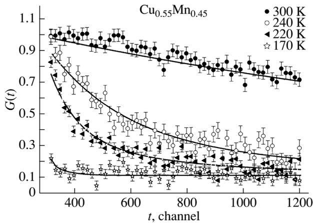
**Fig. 2.** Relaxation functions for the  $\text{Cu}_{0.55}\text{Mn}_{0.45}$  sample at different temperatures in the range 170–300 K. One channel on the time scale corresponds to 0.625 ns. The origin of the scale is located at the 274th channel.
