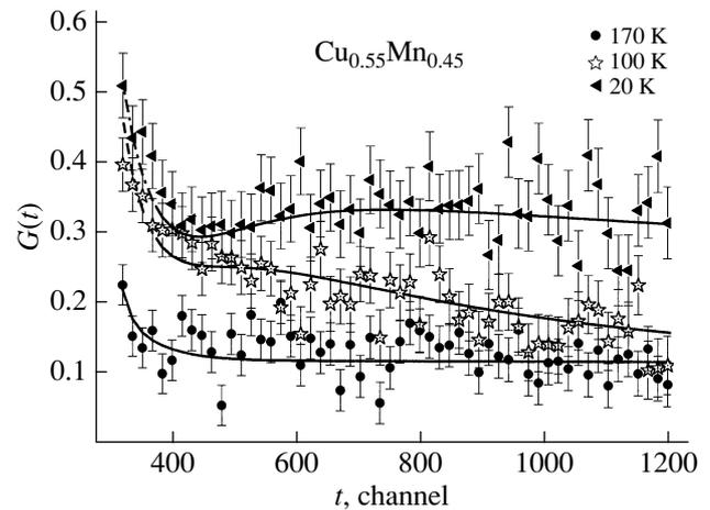
**Fig. 3.** Relaxation functions for the  $\text{Cu}_{0.55}\text{Mn}_{0.45}$  sample at different temperatures in the range 20–170 K. One channel on the time scale corresponds to 0.625 ns. The origin of the scale is located at the 274th channel.
