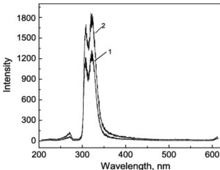
**Fig. 5.** X-ray induced emission spectra: 1 – BaF<sub>2</sub>:Ce (0.1 %) single crystal and 2 – BaF<sub>2</sub>:Ce (0.1 %) ceramics
