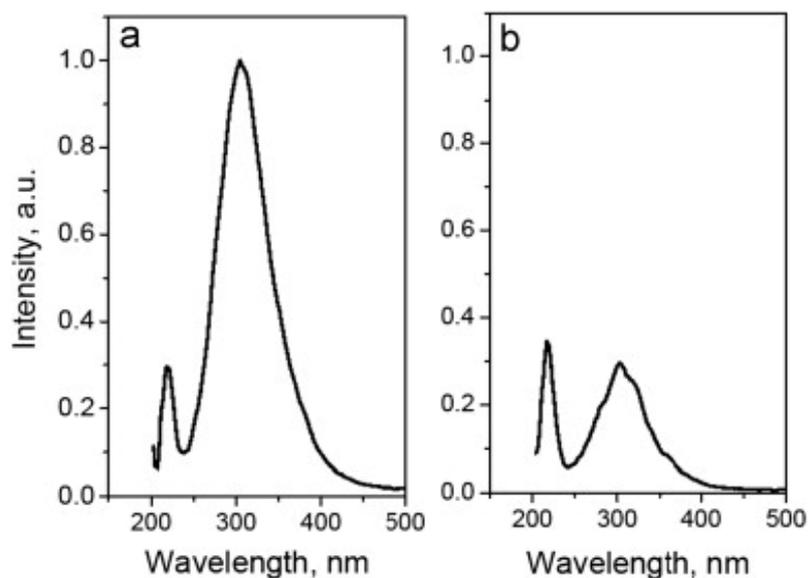
Fig. 2. X-ray luminescence spectra of a single BaF<sub>2</sub> crystal (a) and of ceramics (b)
