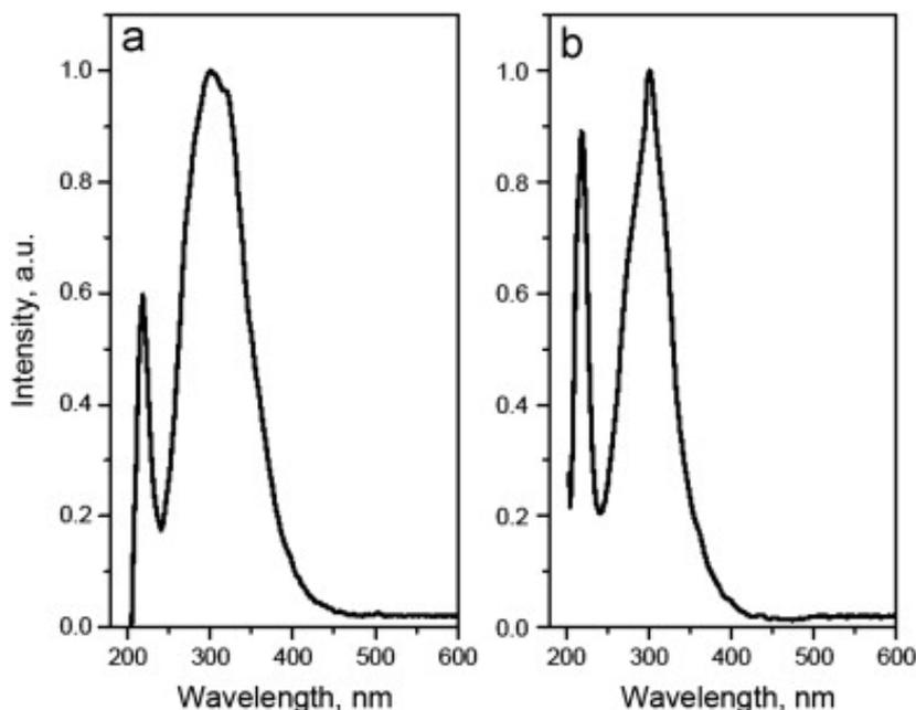
**Fig. 3.** Light yields of a single BaF<sub>2</sub> crystal without annealing in CF<sub>4</sub> (a) and of a BaF<sub>2</sub> crystal doped by 1%ScF<sub>2</sub> with annealing in CF<sub>4</sub> (b)
