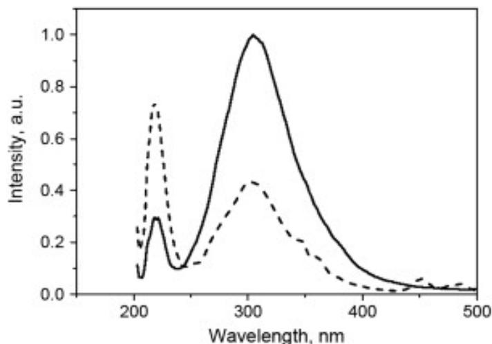
**Fig. 4.** X-ray luminescence spectra of a single BaF<sub>2</sub> crystal (solid line) and a crystal of BaF<sub>2</sub> doped with Tm (dash line). The BaF<sub>2</sub>:0.5%Tm crystal has the light yield of the 0.9 ns component 2.4 times larger than that of a single BaF<sub>2</sub> crystal and the slow component yield smaller by the same factor
