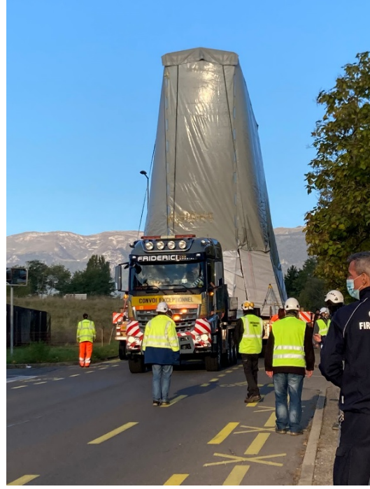
Fig. 7. Installation of the last sector on the disk of the NSW C detector ( left ). Transport of the NSW C detector from the assembly area to the ATLAS experiment shaft ( right )
