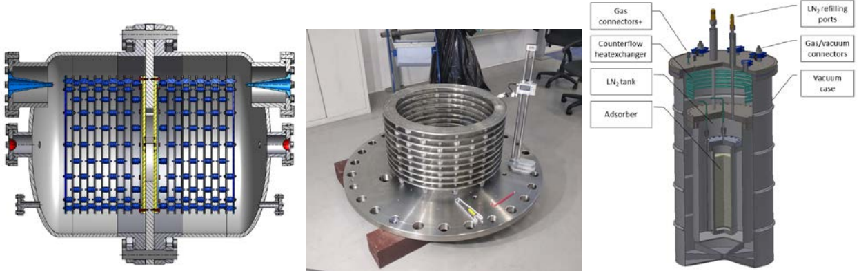
Fig. 11. A drawing of two-cell variant of a high-pressure TPC ( left panel ); a test assembly of the TPC inner structure ( middle panel ); a design of the gas purification unit ( right panel )
