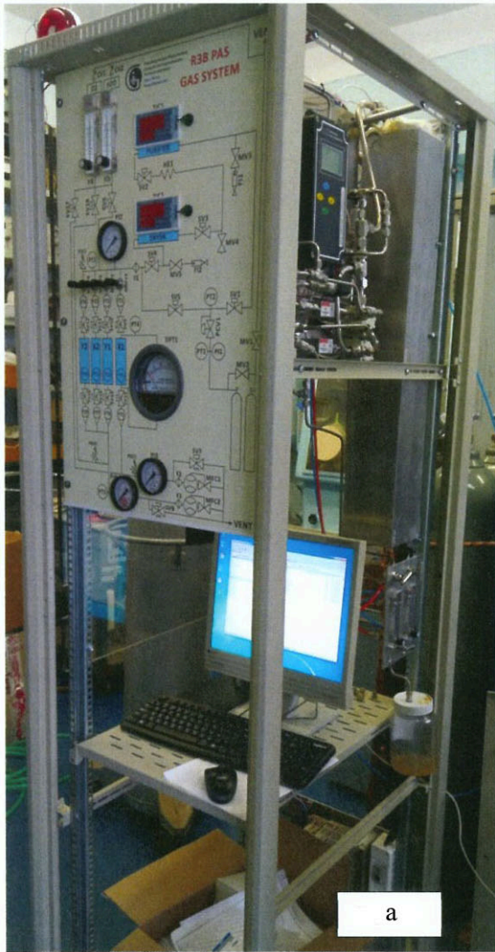
Fig. 6. Proton arm spectrometer gas supply system appearance (a) and system software main window (b); pressure stabilization in X1 plane (PT4) and in X2, Y1, Y2 planes (PT5) (c)
