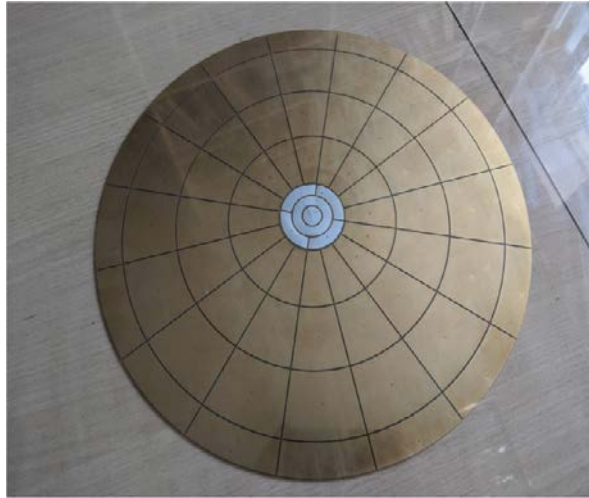
Fig. 7. The ACTAF2 segmented anode plane with the central Kapton part
