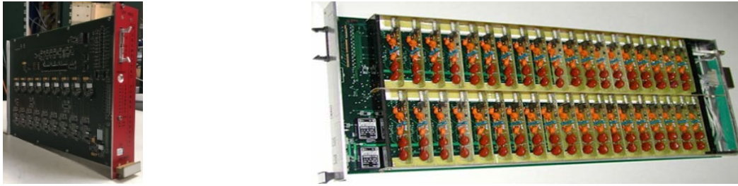
Fig. 3. High voltage segmented power supply modules ( left ) and distribution boards DB36 ( right )
