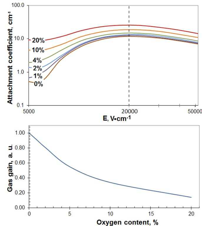
**Fig. 3.** Electron attachment coefficient as a function of the electric field strength (*top*); the gas gain as a function of the oxygen content (*bottom*)
