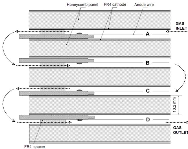
**Fig. 1.** Cross section of the LHCb muon chamber
