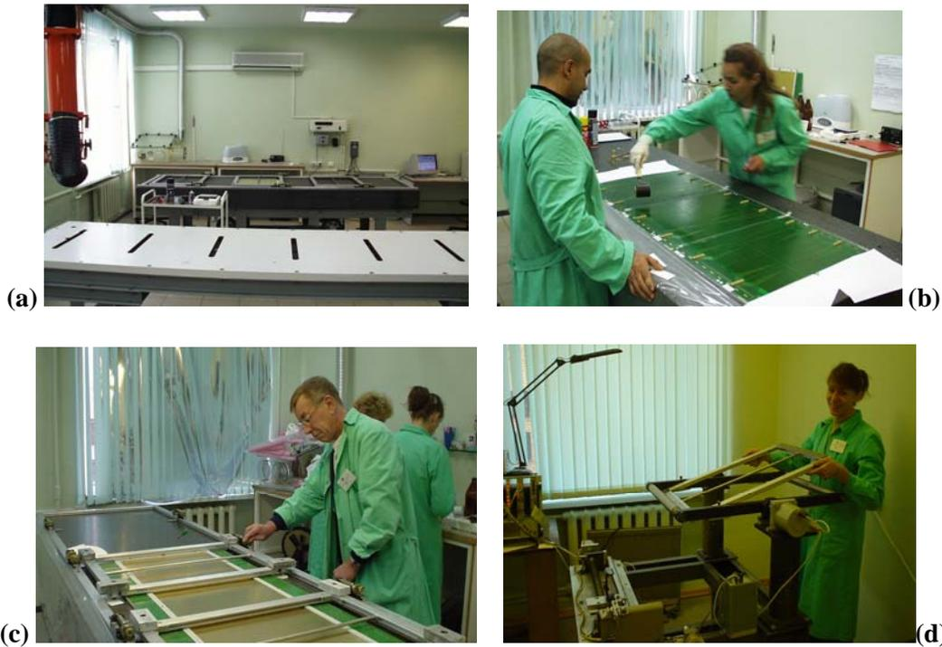
**Fig. 7.** A view of clean assembling room (a), gluing of the PCB to the composite sandwiches (b), wiring machine (d), and installation of the signal wires on a wire plane (c)
