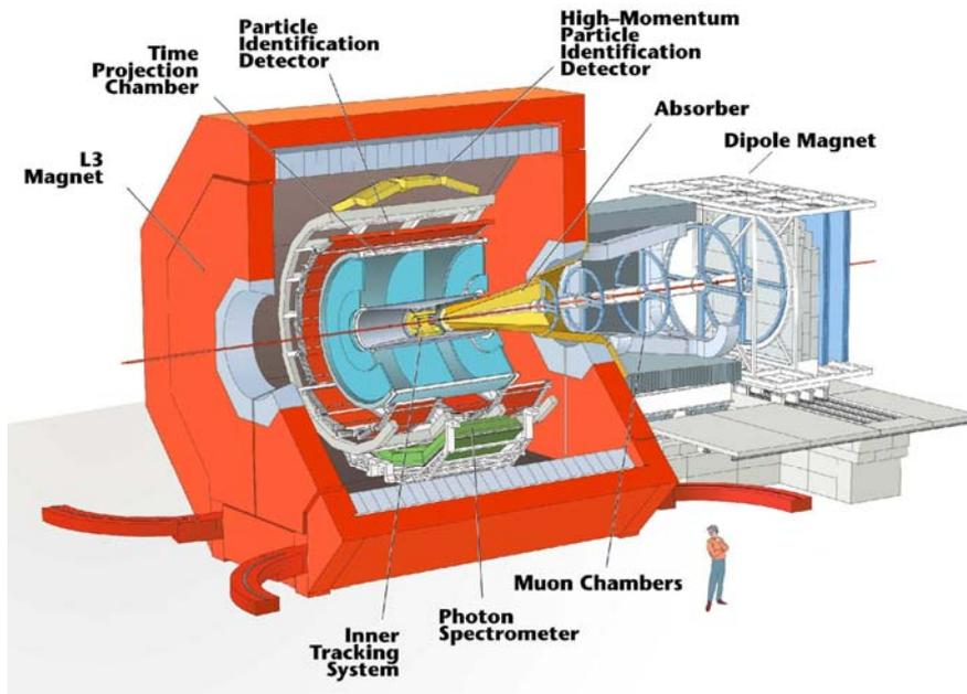
Fig. 1. The layout of the ALICE detector. The muon spectrometer arm is depicted on the right side of the figure
