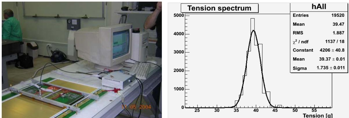
**Fig. 5.** The equipment for wire tension measurement and the wire tension distribution measured for about 20,000 wires in the chambers produced at PNPI
