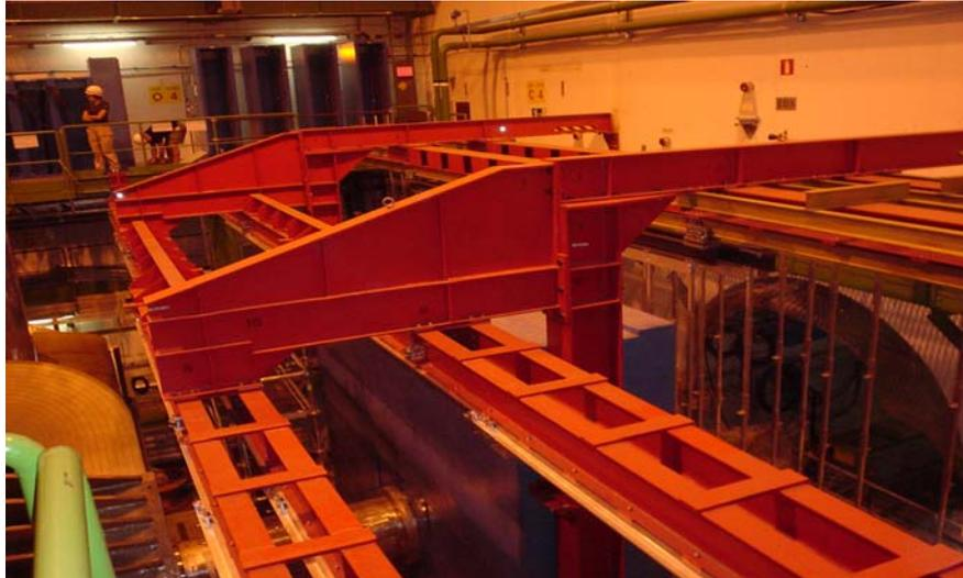
**Fig. 9.** Superstructure for support of the tracking and trigger chambers designed by the PNPI group
