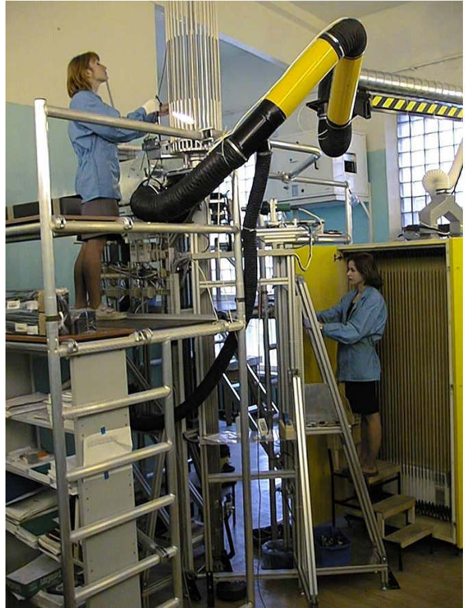
Fig. 2. View of Straw Reinforcement Machine at PNPI
