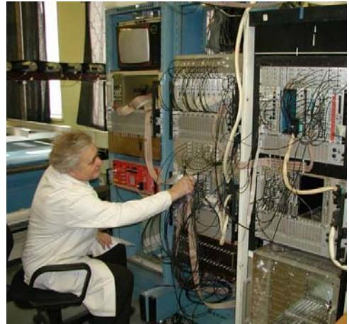
**Fig. 6.** Final tests of the muon chambers on the cosmic ray test stand
