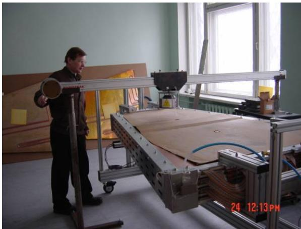
**Fig. 3.** Muon chamber on the  $\gamma$ -rays test stand
