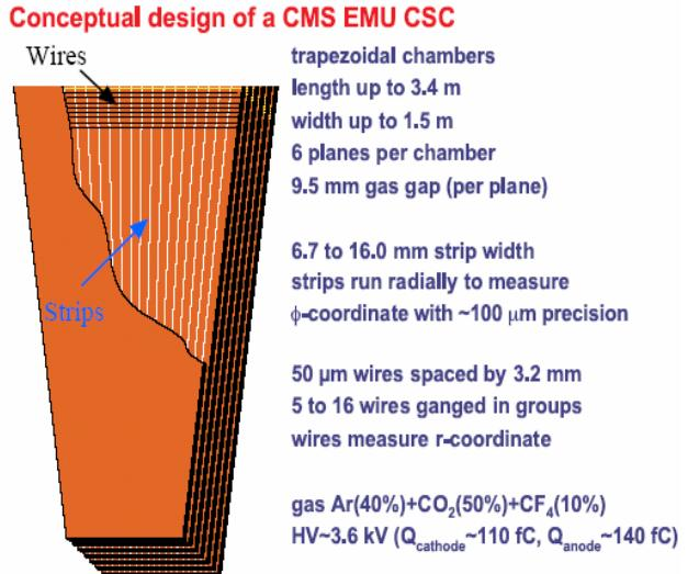
**Fig. 2.** Sketch view and some parameters of a CSC
