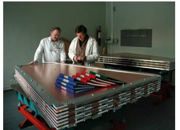
**Fig. 4.** Muon chamber ready for installation of the on-chamber electronics
