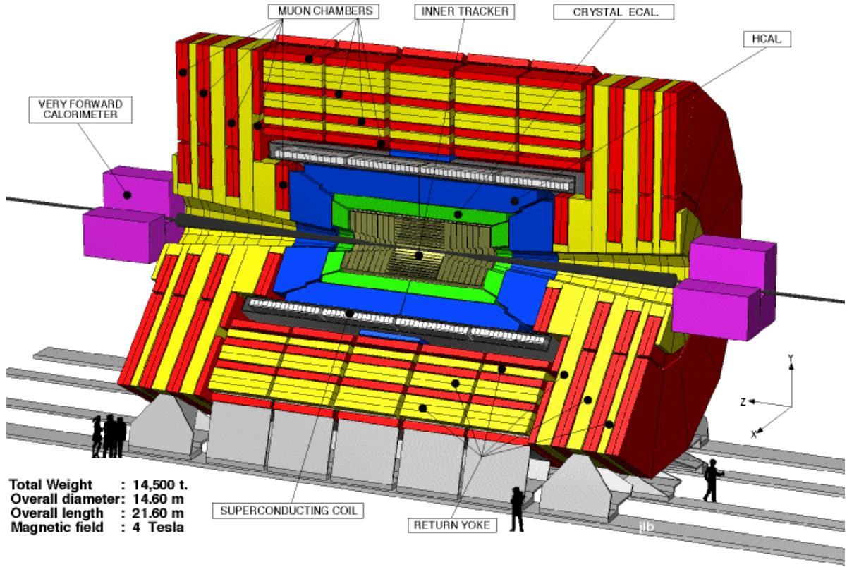
**Fig. 1.** General view of the CMS detector
