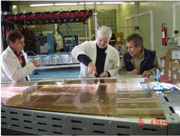
**Fig. 5.** Installation of the on-chamber electronics
