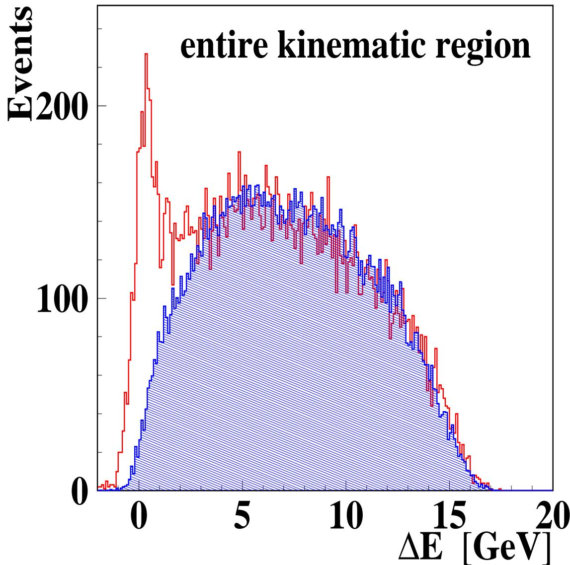
$\Delta E = \frac{M_X^2 - M_p^2}{2M_p}$ .  $M_X$  and  $M_p$  are masses of recoil system and proton, respectively.
