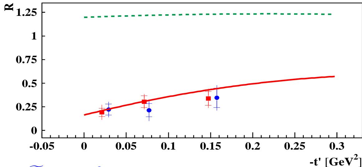
$$R = \frac{\sum_{\lambda\omega} |F_{\lambda\omega 0}|^2}{\sum_{\lambda\omega} |F_{\lambda\omega 1}|^2} \approx \frac{1}{\epsilon} \frac{r_{00}^{04}}{1-r_{00}^{04}} \approx |T_{00}|^2 / [|T_{11}|^2 + |U_{11}|^2].$$
