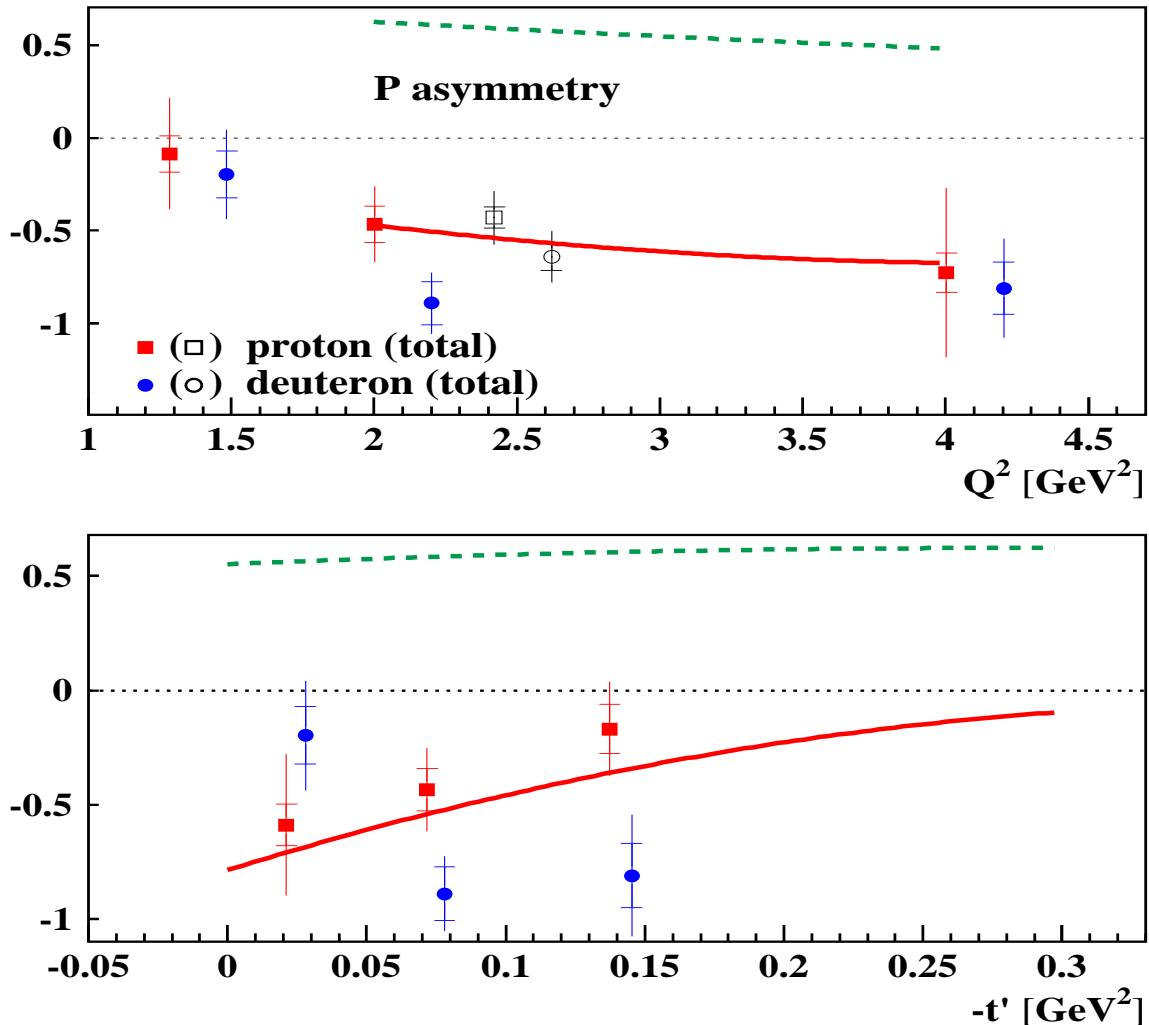
$$P = \frac{d\sigma_T^N - d\sigma_T^U}{d\sigma_T^N + d\sigma_T^U} \approx \frac{2r_{1-1}^1 - r_{00}^1}{1 - r_{00}^{04}}$$
