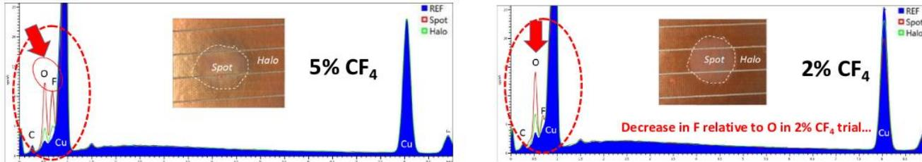
Anode surface: visually dark in the area irradiated with 2% CF<sub>4</sub>, confirmed with SEM. Wires irradiated with 5% CF<sub>4</sub> look similar to the reference non-irradiated wires.
