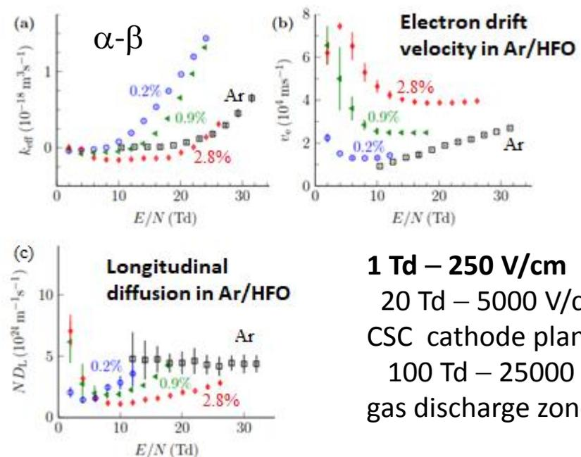
Figure 8: (a) Effective ionization rate coefficient, (b) electron drift velocity and (c) density normalized longitudinal electron diffusion coefficient in pure Ar and in the mixtures of 0.2%, 0.9% and 2.8% HFO1234ze in Ar as a function of  $E/N$ .
