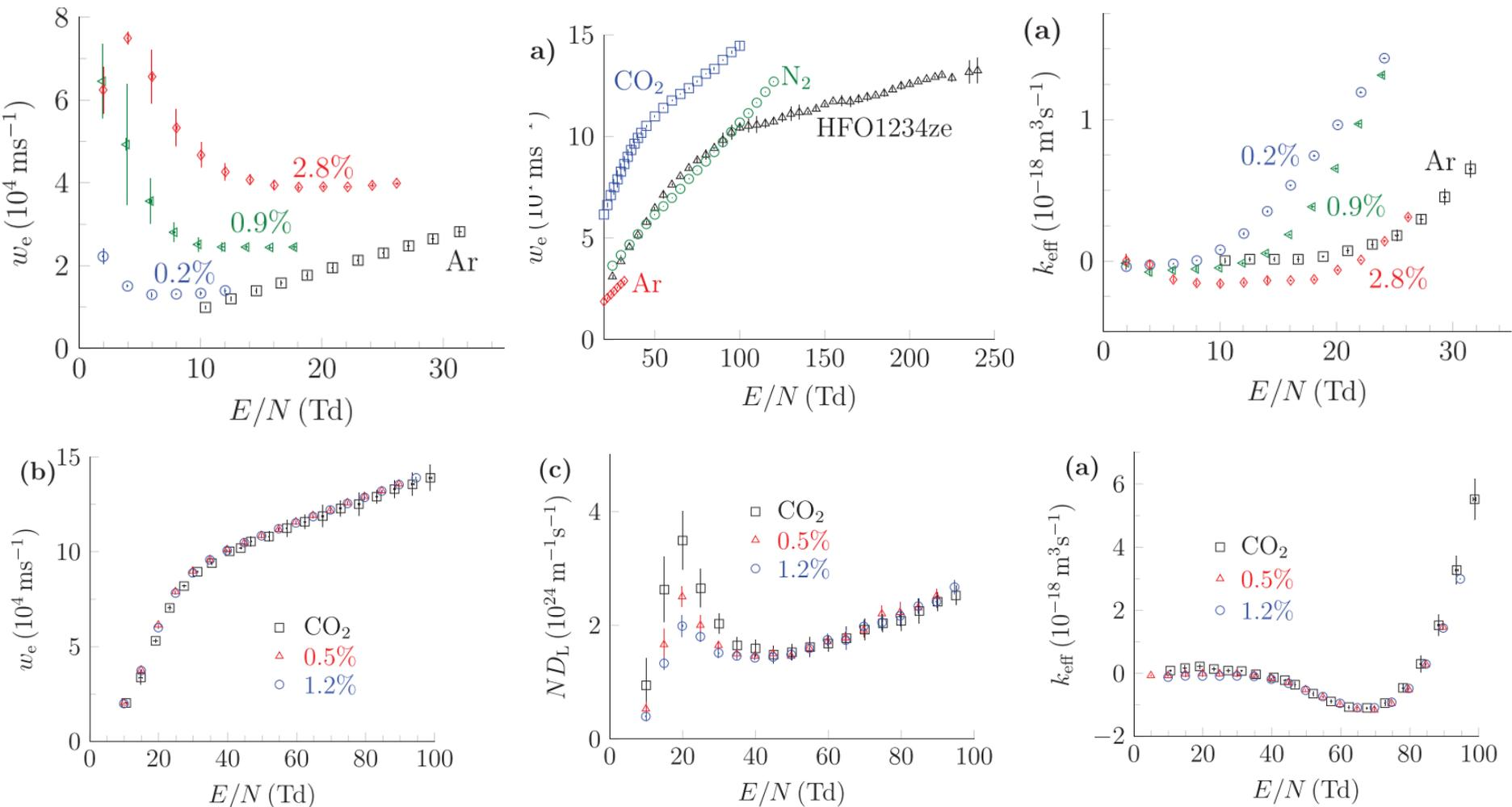
**Figure 7.** (a) Effective ionization rate coefficient, (b) electron drift velocity and (c) density normalized longitudinal electron diffusion coefficient in pure  $\text{CO}_2$  and in mixtures of 0.5% and 1.2% HFO1234ze in  $\text{CO}_2$  as a function of  $E/N$ .
