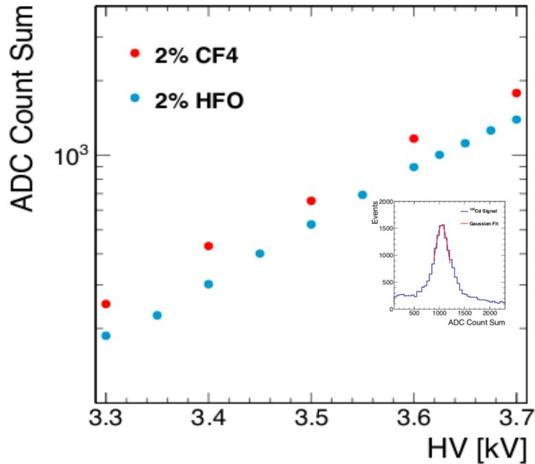
Efficiency plateau measured with  $^{109}\text{Cd}$  source using standard CSC electronics
