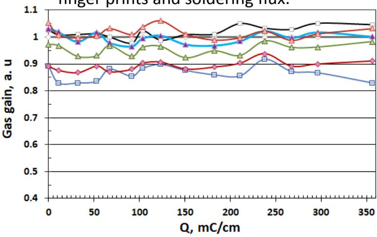
No performance degradation was observed in longevity tests with CSC prototypes in PNPI
