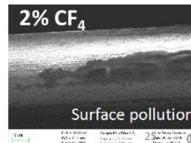
**A definite presence of the dark flakes (Carbon?) on the irradiates wires at 2% CF<sub>4</sub> !!**
