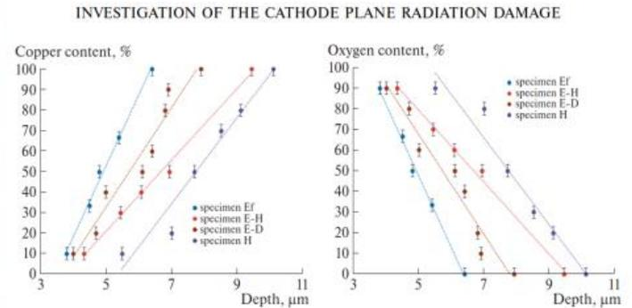
Fig. 9. (Left) copper and (right) oxygen distribution versus depth in copper foil.
