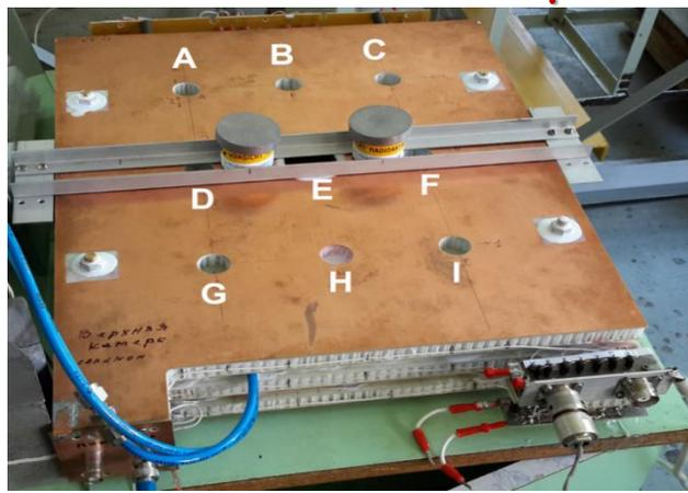
Cathode intently contaminated with RTV, finger prints and soldering flux.
