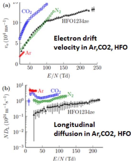
Figure 4: (a) Electron drift velocity  $v_e$  and (b) density normalized longitudinal electron diffusion coefficient  $ND_L$  in HFO1234ze, N<sub>2</sub>, CO<sub>2</sub> and Ar as a function of  $E/N$ .
