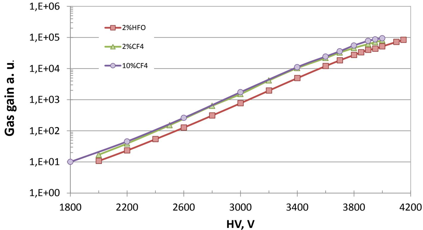
CSC HV working point  $\rightarrow$  Gas gain =  $5 \times 10^4$
