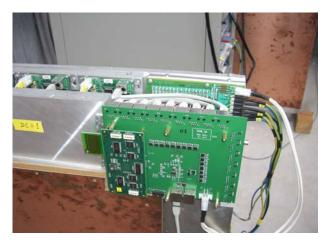
**Fig. 2.** CROS-3 Digitizers and Concentrator are on-chamber mounted system components
