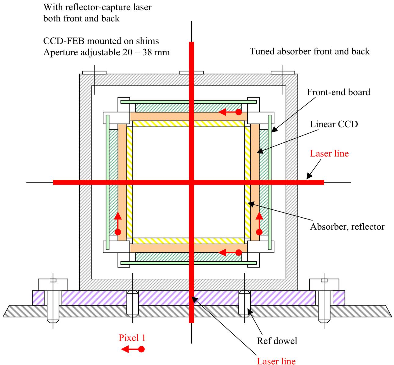
Figure 3. CCD Optical Position Sensor
