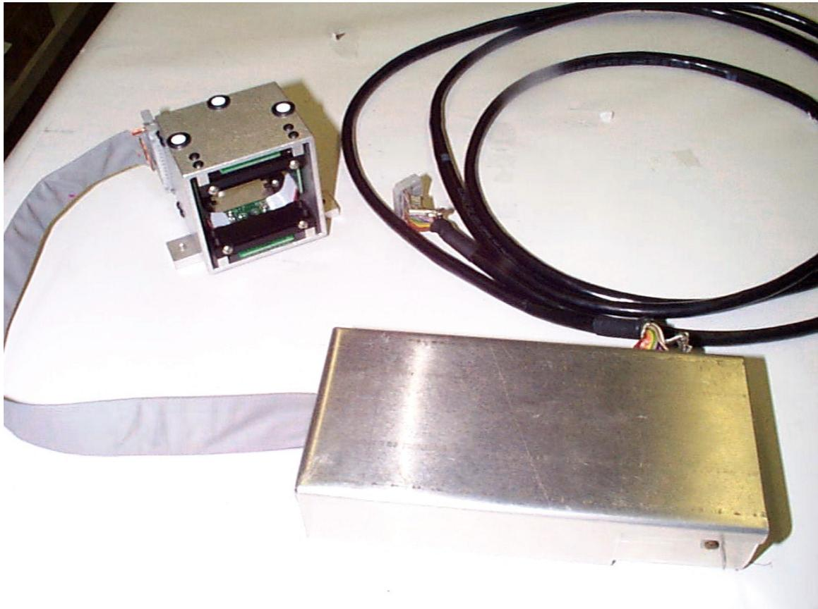
Figure 2. CCD Optical Position Sensor and Digital Readout (DCOPS)
