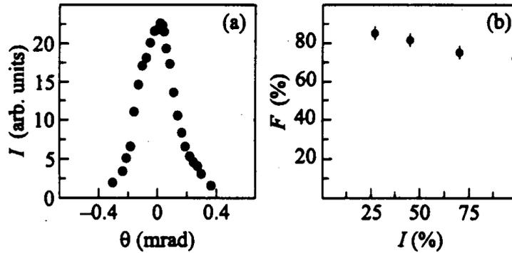
Fig. 9. (a) Dependence of extracted beam intensity on orientation of crystal 1;
