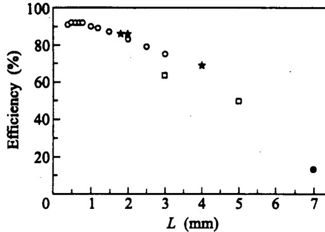
Fig. 11. Crystal extraction efficiency for 70 GeV protons: (\*) – results for S-crystals 1.8, 2.0, and 4 mm, results for O-crystals 3 and 5 mm, (●) – result for S-crystal 7 mm, (o) – Monte Carlo prediction for a perfect crystal with 0.9 mrad bending
