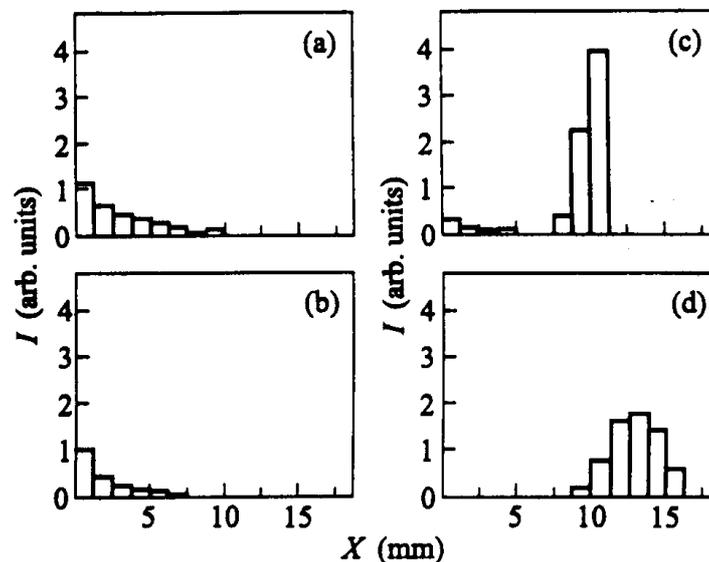
Fig. 10. Beam profiles measured on the collimator entry face: (a) crystal is out, beam scraped by collimator alone; (b) crystal is in the beam, but misaligned; (c) crystal is in the beam, aligned; (d) crystal is out, beam kicked by magnet
