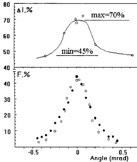
**Fig. 7.** Bottom: the extraction efficiency as a function of the crystal angle; the measurements (open circles) and simulations (dots). Top: the reduction in the beam store as a function of the crystal angle under conditions of a feedback system
