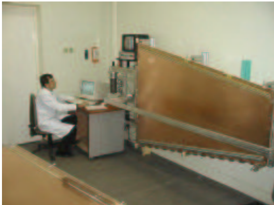
Fig. 8. Wire pitch and tension control
