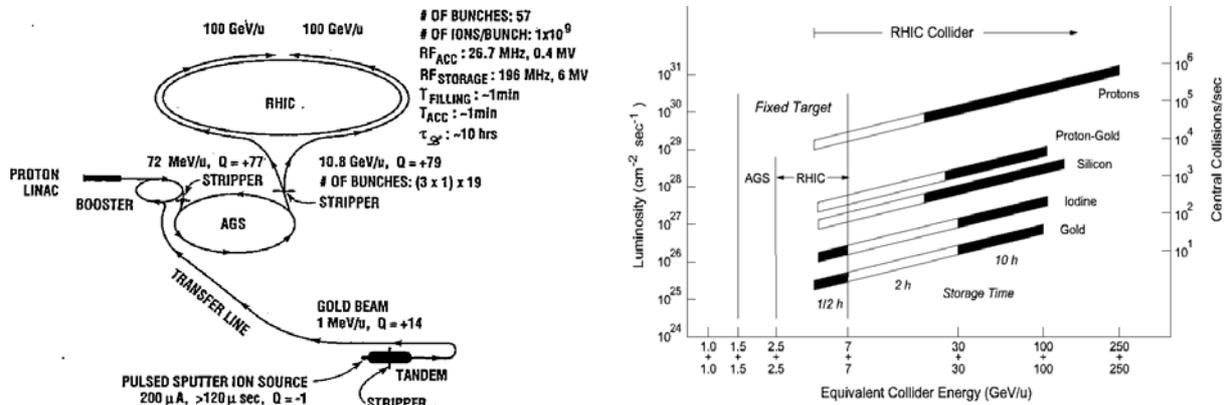
Fig. 1. RHIC accelerator complex at BNL (left). The RHIC luminosity and number of central collisions per second for impact parameters less than 1 fm (right)
