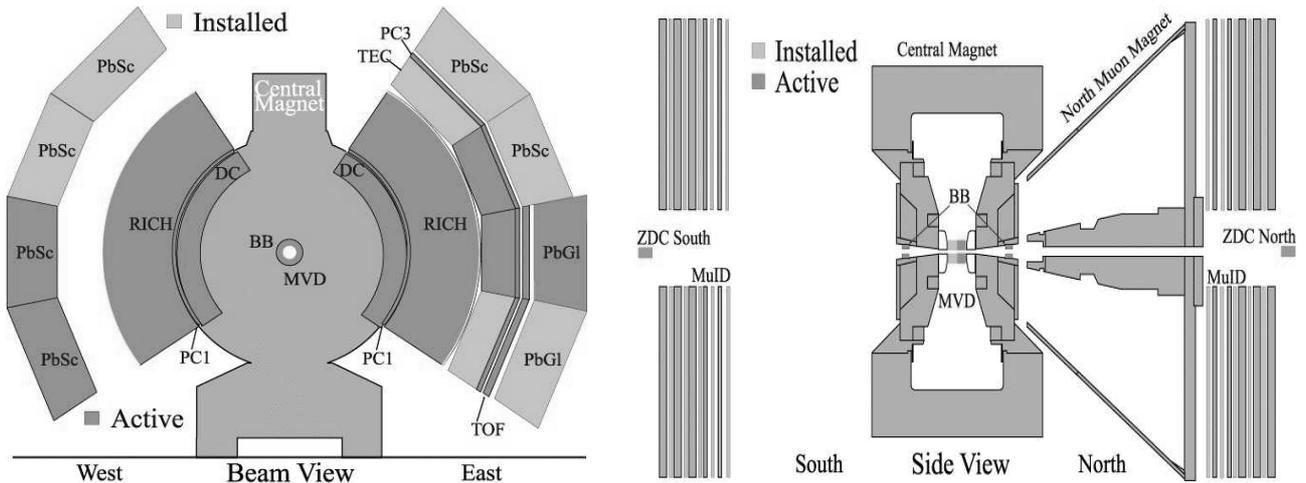
Fig. 3. Detectors installed/active for the first run of RHIC in summer of 2000
