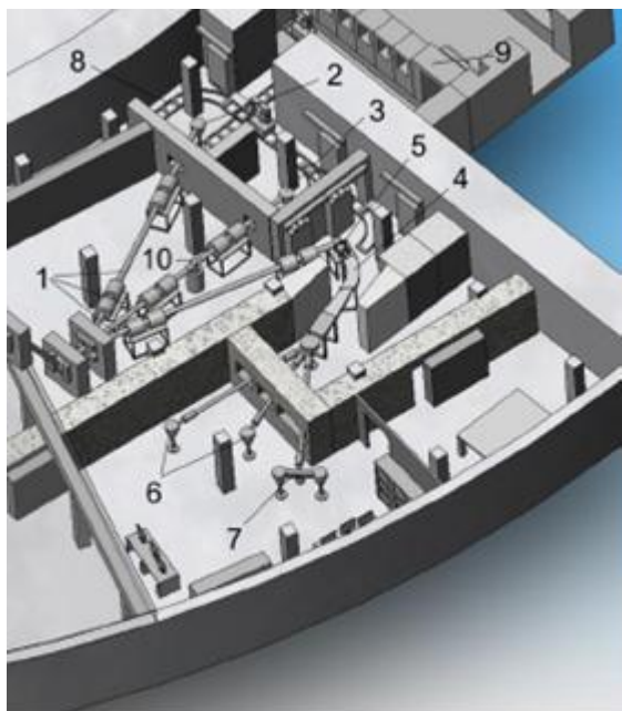
Fig. 1. Layout of RIC-80 radioisotope complex. 1 – proton beam lines to target stations (cellar), 2 – target station for radiochemical extraction of produced isotopes, 3 – target station for dry (high temperature heating) extraction of produced isotopes, 4 – mass-separator for production of medical isotopes samples of a high purity, 5 – target station of mass-separator, 6 – collecting stations for separated radio- nuclides, 7 – detector stations for obtained radionuclide purity measurement, 8 –
