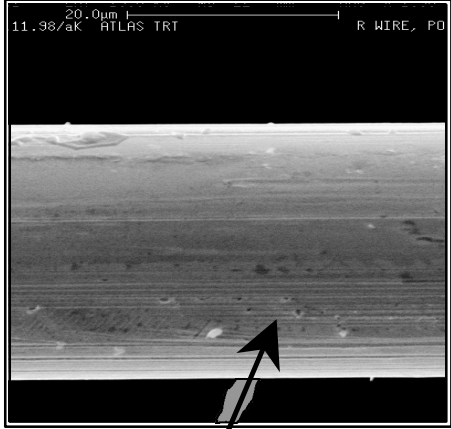
Fig.2a. Edge of the wire. Non-irradiated zone. Diameter - 35 \mu\text{m} .
