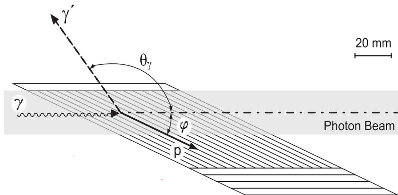
**Fig. 3.** Top view on a multi-strip anode: the 2 cm broad photon beam enters the volume of the IC from the left side. In the case a photon is scattered under the angle  $\theta = 130^\circ$ , the scattered proton gets a momentum along an anode strip (at  $\phi = 22^\circ$ )
