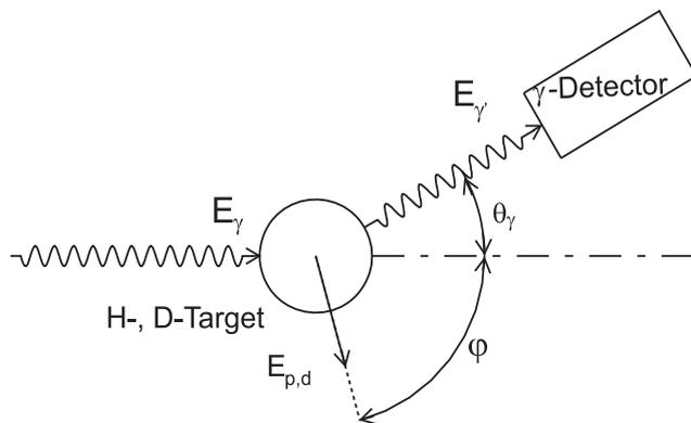
**Fig. 1.** Experimental method (schematic). A photon beam with a full bremsstrahlung spectrum is scattered from a gaseous hydrogen/deuterium target inside a high pressure ionization chamber, the energy of the scattered photons is determined in a  $\gamma$ -detector under a certain angle. By detecting the scattered bremsstrahlung photon in coincidence with the recoiling proton (deuteron) in the ionization chamber the incoming photon energy is determined
