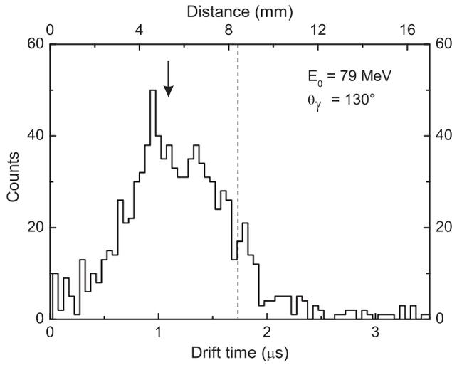
**Fig. 6.** Drift-time distribution of proton signals in an IC. The dashed line denotes the centre of the active volume between electrodes. The actual location of the photon beam is indicated by the arrow
