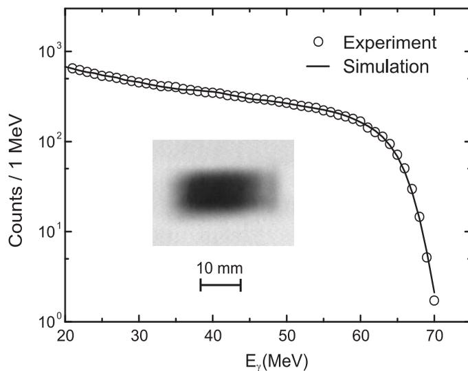
**Fig. 2.** Bremsstrahlung spectra and a part of a colour inverted Polaroid picture of the collimated bremsstrahlung beam approximately 3 m behind the bremsstrahlung target: Areas with high beam intensity are dark, with low intensity are grey. Circles correspond to the measured bremsstrahlung spectrum. The curve shows a folded simulation spectrum
