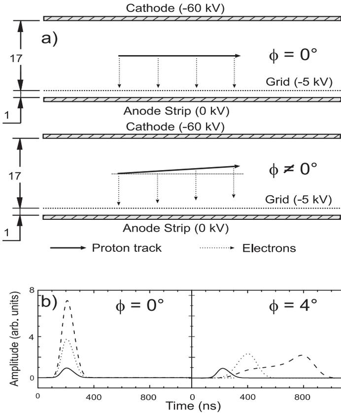
**Fig. 4.** a – side view of the chamber electrodes. The upper part shows a track of a proton, parallel to the anode. The lower part demonstrates a track of a proton under a finite angle. Dimensions are in mm; b – simulated pulse form for different azimuthal angles and for different proton energies: 1 MeV (solid line), 4 MeV (dotted line) and 8 MeV (dashed line)
