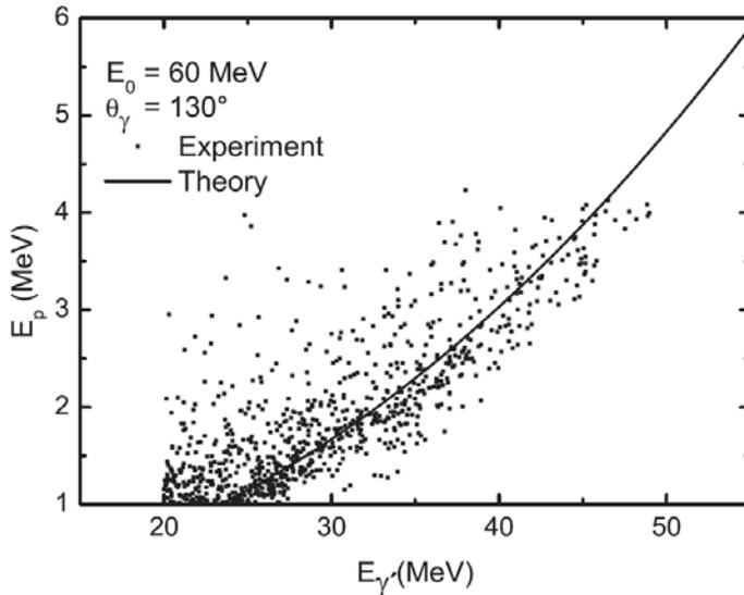
**Fig. 7.** Measured energy correlation of the scattered photons ( $E_\gamma > 20$  MeV) and recoil protons ( $E_p > 1$  MeV) in comparison with the expected kinematic relation for  $E_\gamma$  and  $E_p$  (solid curve) for the data taken at  $E_0 = 60$  MeV and  $\theta = 130^\circ$ . The proton recoil energies are determined from the measured charges, collected on the IC anodes, with the help of Eq. (1)
