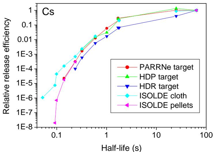
**Fig. 4.** Comparison of the Cs yield trends from HDR, HDP, LDP PARRNe IRIS and ISOLDE targets. The yields are normalized at the yield point of <sup>140</sup>Cs with the half-life  $T_{1/2} = 63.7$  s
