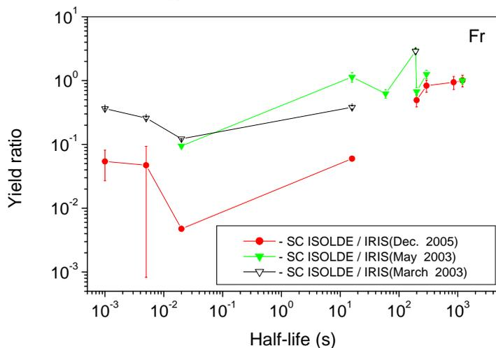
**Fig. 5.** Ratio of the yields of Fr isotopes from ISOLDE graphite-cloth target to the yields of the same isotopes from HDR (triangles) and HDP (circles) targets, plotted as a function of the half-lives. The obtained ratios are normalized at the point <sup>212</sup>Fr with the half-life  $T_{1/2} = 20$  min
