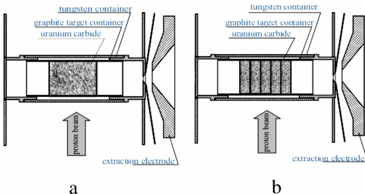
**Fig. 1.** Schematic drawings of a) high density rod (HDR) uranium carbide target; b) high and low density pellet uranium carbide target
