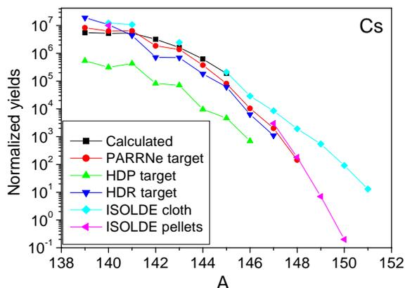
**Fig. 2.** The yields of Cs isotopes released from a high density rod, high density and low density pellet targets at  $2100^\circ\text{C}$ . The yields from ISOLDE  $\text{UC}_x$  pellet target are presented. The yields calculated on the basis of measured cross section are shown as well
