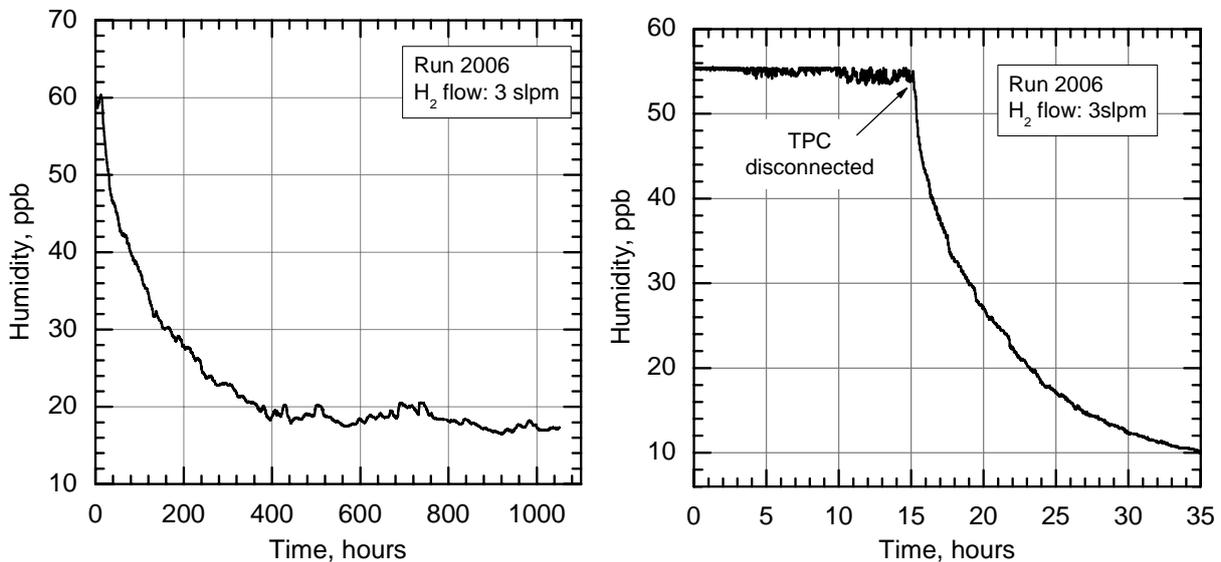
Fig. 4. Humidity decrease in the TPC after CHUPS connection (left) and after bypassing the TPC (right)
