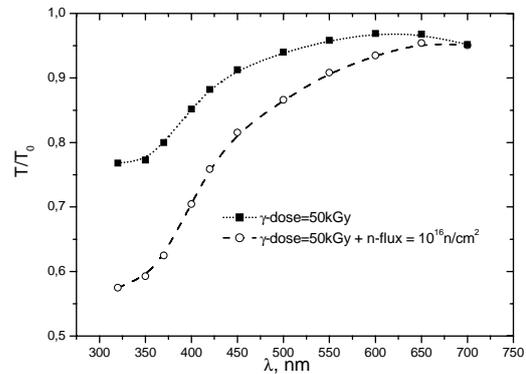
**Fig. 4.** Relative transmittance  $T/T_0$  for a  $\gamma$ -dose of 50 kGy and neutron irradiation with fluence of  $10^{16}$  n/cm<sup>2</sup>
