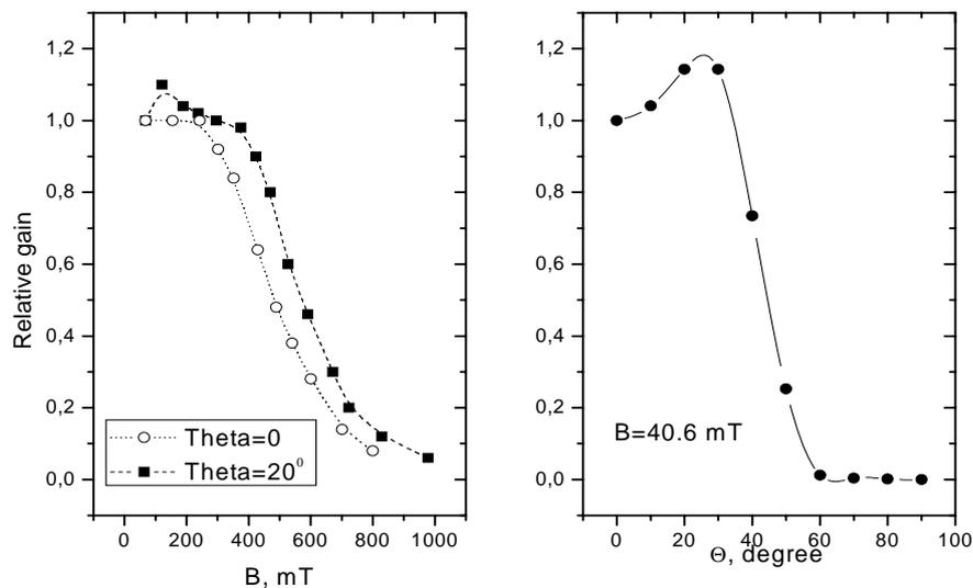
Fig. 8. Magnetic properties of fine-mesh FEU-187
