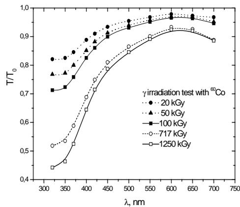
Fig. 2. US-49 relative glass transmittance for different of gamma radiation doses at <sup>60</sup>Co gamma facility
