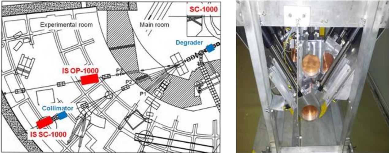
**Fig. 1.** Scheme of the proton beam lines: P2 – protons with the energy of 1 000 MeV; P3 – protons with the energy variable from 1 000 to 60 MeV (*left*); device for remote variation of the absorber length and of the proton energy (*right*)
