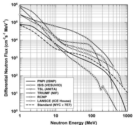
**Fig. 3.** General layout of the neutron time-of-flight spectrometer GNEIS and IS NP test facility (left); neutron spectrum  $F_{IS NP}(E)$  of the IS NP/GNEIS facility in comparison with the standard terrestrial neutron spectrum and spectra of other world-class test facilities (right)
