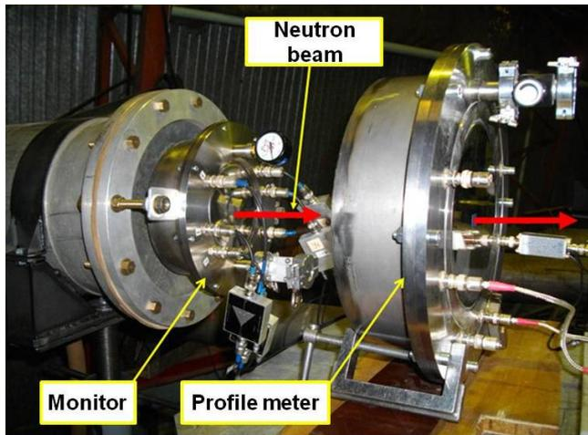
Fig. 4. Neutron monitor and a profile meter MWPC
