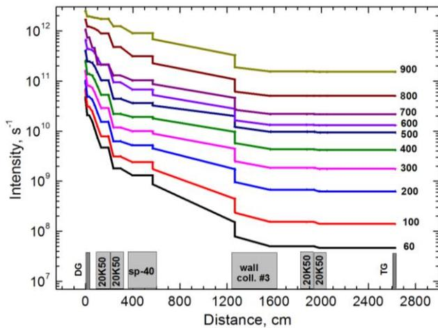
**Fig. 2.** Dynamics of protons losses at different energies along the beam line P3: DG – absorber; 20K50 – quadrupole; SP-40 – bending magnet; wall, coll. #3 – a wall with the collimator #3 between the main and experimental room of the accelerator; TG – target
