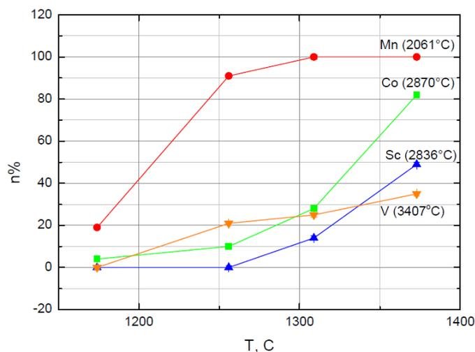
**Fig. 6.** The evaporated fractions of different radionuclides produced by nuclear reactions in the copper target material and evaporated from it at different temperatures [6]. In the right side in brackets, the boiling points of the evaporated species are presented
