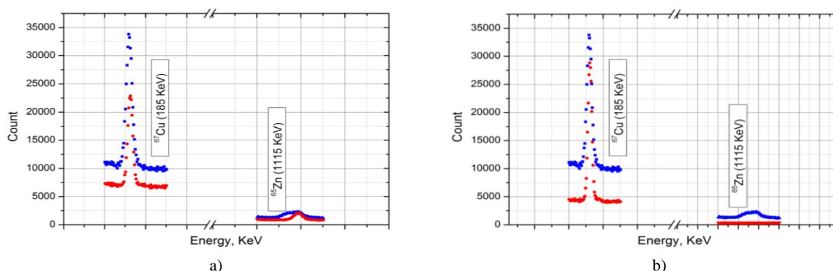
**Fig. 4.** The spectrum of the vessel with the irradiated Zn before heating is shown by *blue dots*; the spectrum after one hour vessel heating at a temperature 700 °C is shown by *red dots* (a). The spectrum of the evaporated copper atoms collected at the cold finger cooled by floating water after the vessel heating at a temperature 1460 °C for two hours is shown by *red dots*; for comparison, the spectrum of the vessel with the irradiated Zn before heating is shown by *blue dots* (b)
