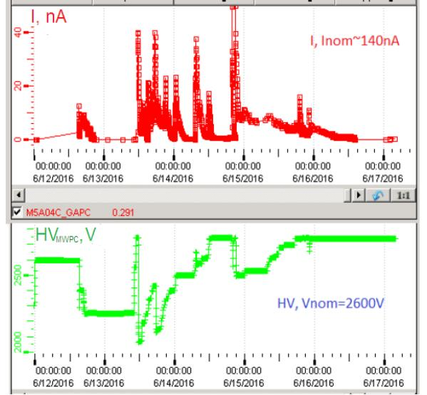
**Fig. 2.** Typical recovery procedure from the ME at the beam
