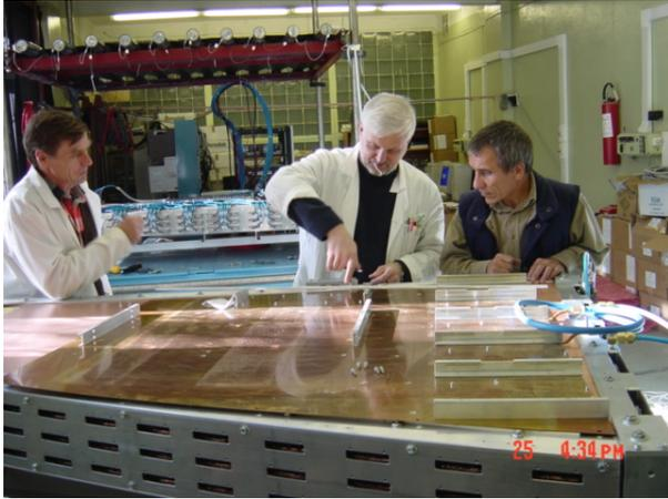
**Fig 5.** Installation of the on-chamber electronics
