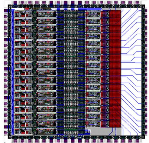
Fig. 17. CMP16 (Bondar's chip) layout
