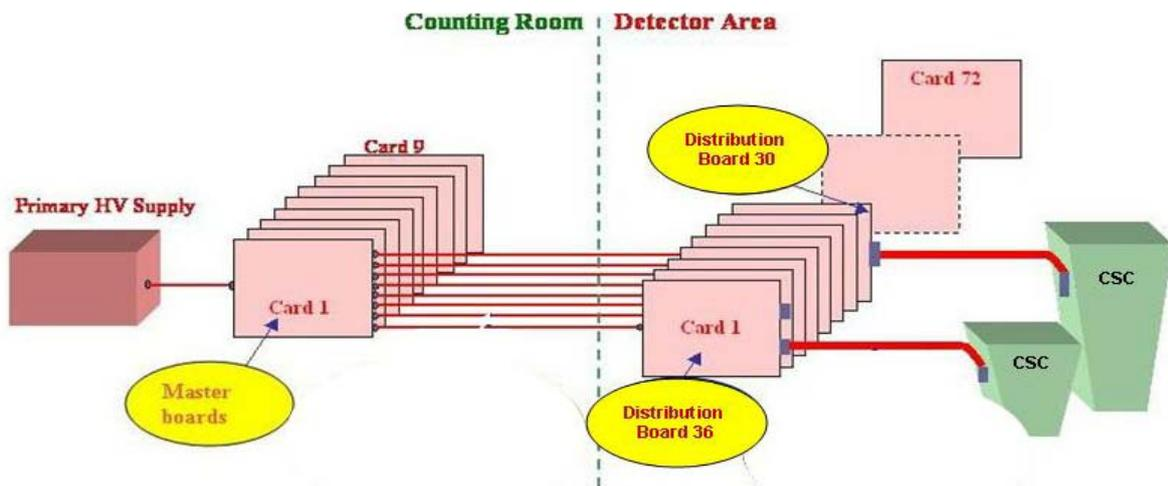
Fig. 13. Block diagram of a quarter of EMU HV system
