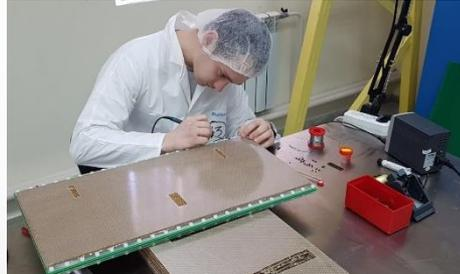
Soldering HV connector and readout pins
