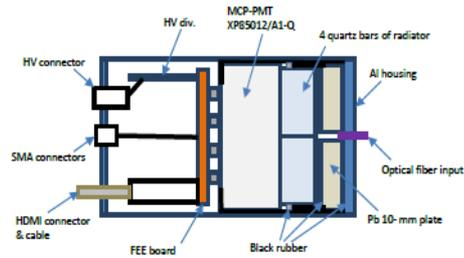
Fig. 4-1. A scheme of the FFD module.
