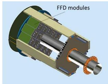
The FFD sub-detector consists of 20 modules based on Planacon multianode MCP-PMTs
