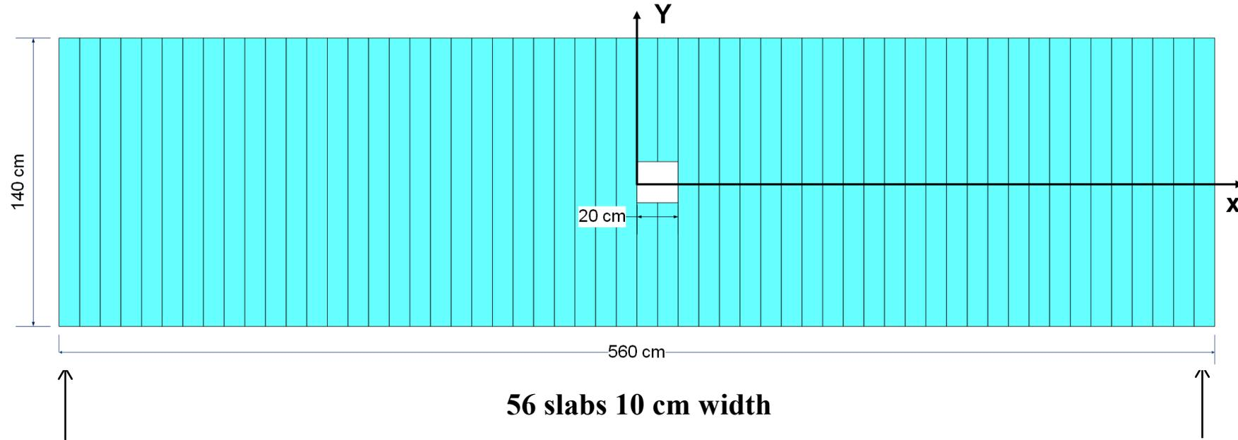
Comment. The beam pipe diameter at this z-location is 180 mm. i.e. 2 slabs to be cut.
