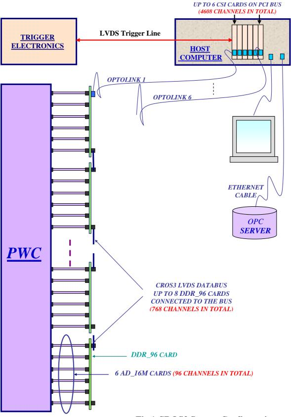
Fig.1 CROS3 System Configuration
