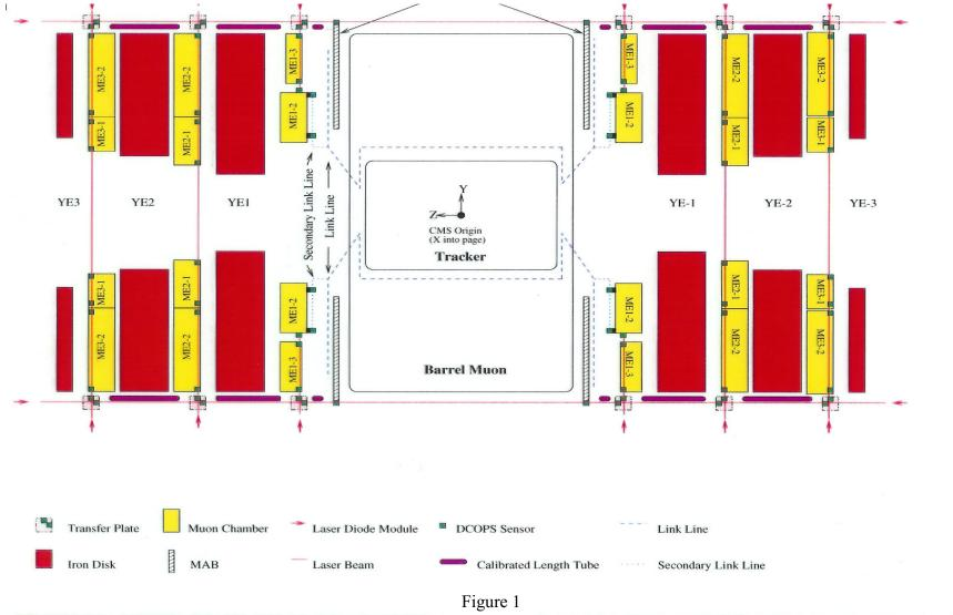
SECTION VIEW OF EMPMS TRANSFER LINE AND SLM LINE CONNECTION OF CSC LAYERS
