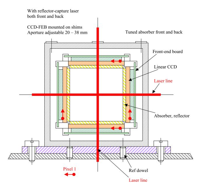
Figure 3. CCD Optical Position Sensor
